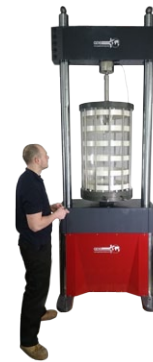
Traditional passive triaxial cell in 250kN load frame (300TC/1)
