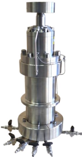
32MPa triaxial cell with balanced ram 54mm max sample diameter
