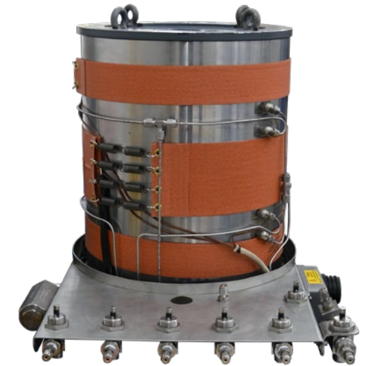
Instrumented Hoek Cell, shown with heat pads (GDSHC)
