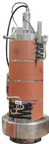
20MPa triaxial cell with heating pads 100mm max sample diameter
