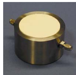
Fig. 1 HAEPD bonded into a standard triaxial pedestal
