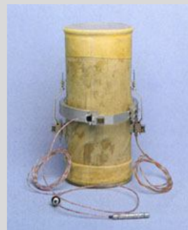
Fig. 12 Hall Effect and LVDT local strain transducers
