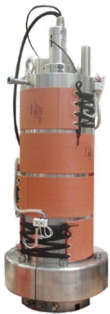
Heating only temperature bands.
