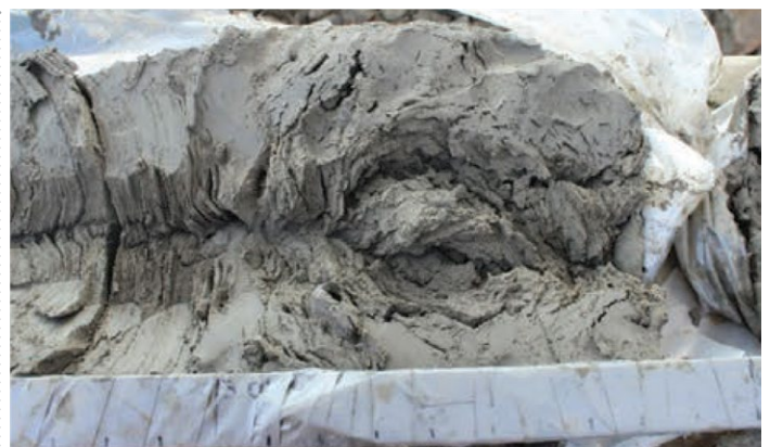
Figure 3: Photo of Upper GLU soil sampled from within the breach area, showing contorted and folded laminations.
