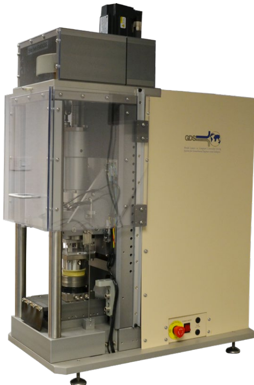
Figure 4: GDS Instruments Electromechanical Dynamic Cyclic Simple Shear Device (EMDCSS).
