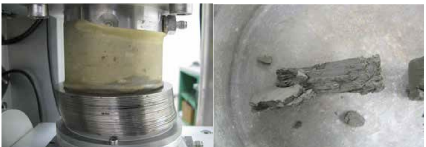
Figure 6: Direct simple shear response and photos of an Upper GLU soil specimen tested under constant volume conditions within a GDS Electromechanical Dynamic Cyclic Simple Shear (EMDCSS) device.
