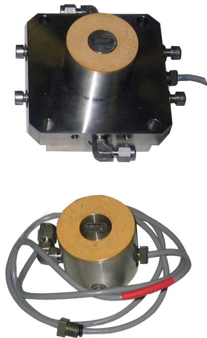
Figure: 5 Bender Element shown in pedestal and topcap.
